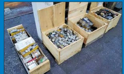
Tooling for Deep Hole Boring Lathes
