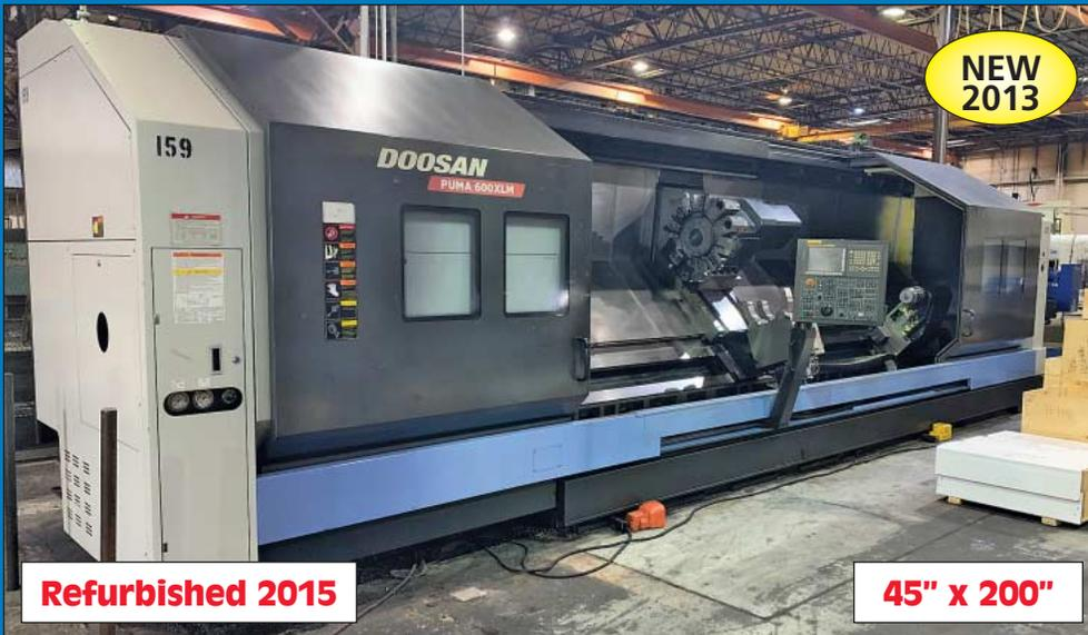
Doosan Puma 600XLM CNC Turning Center, Milling
